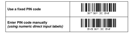
If you want to use a different PIN code or you are only allowed to enter a random PIN code on your OPR3301, then you will have to enter this PIN code using so called direct input labels. These labels can be found below and in the Universal Menu Book (chapter 4.3.3.). After scanning the PIN code, read the END label to send the PIN code to the remote device.
