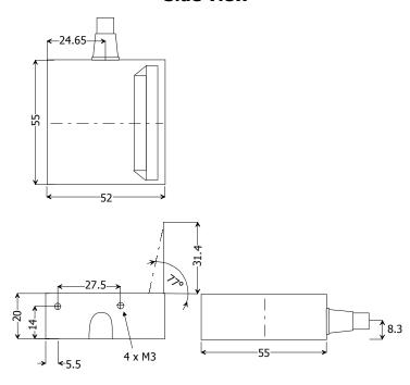
Note: To prevent infiltration of dust or other contaminants into the scanner through the mounting holes provided in the unit's case, short screws (M3-6) may be placed in each hole location. The shafts must not penetrate into the case further than 0.25 inches (6mm).
