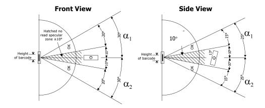
Recommended operation at  $10^{\circ} \le \alpha_{1}$ ,  $\alpha_{2} \le 15^{\circ}$ . Avoid specular reflection dead zone (hatched).
