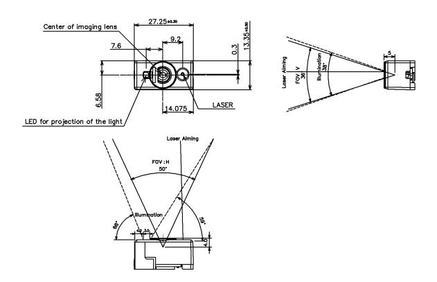
Install the window with sufficient clearance for FOV, Illumination, Laser Aiming.
