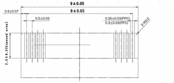
Note 1: Polyimide and a thermally hardened adhesive is recommended as the materials for the stiffener. Note 2: Then using FFC, confirm the tolerance of the FFC thickness coupled to the connector.
