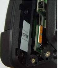
Figure 6-2 Insert SIM card
