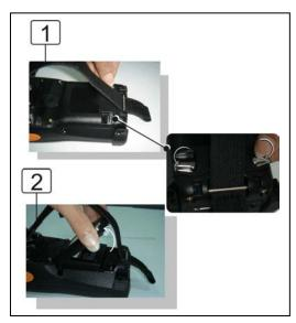
Figure 2-8 Detach the battery cover from PDT
