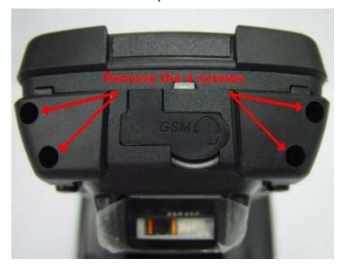
Figure 6-1 Remove screws from End Cap
