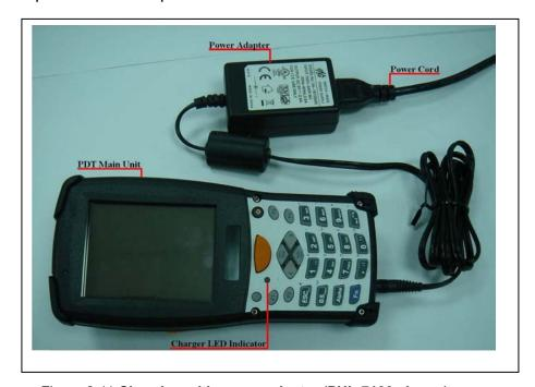
Figure 2-11 Charging with power adapter (PHL-7100 shown)
