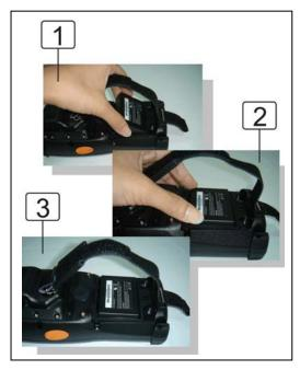
Figure 2-9 Insert the battery pack
