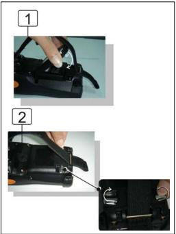
Figure 2-10 Replace the battery cover
